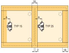
• an example of the use of locks 750.15 and 750.25 (the same distance between the lock and the edge of both full overlay and half overlay cabinet doors)
