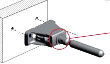
Triade Maxi has to be installed with the arrow facing upwards.
