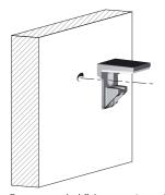
Recommended fixing countersunk screw type - head  $\varnothing$  5 mm max.
