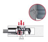
Press strongly with PZ2 cross screwdriver to slot the pinion screw in.
